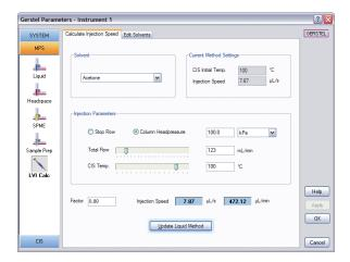
The LVI Calculator is an integral part of the MAESTRO Software. After selecting the solvent from a pull-down menu and entering the injection volume and column flow, a set of optimized method parameters are suggested, which can be transferred to the method by mouse click.
