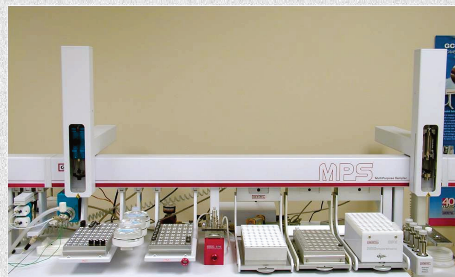
Figure 2. MPS XL Multi-Purpose Sampler with the GERSTEL DPX option for extraction of mycotoxins.
